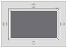
Make sure to leave adequate space around the screen for ventilation purposes. Do not cover the ventilation holes on the rear, as this may cause the screen to overheat
