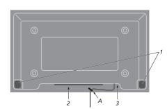
For safety reasons, you must secure the mains lead in the cable clamp (A). Otherwise, the mains cable can be tugged free of the socket.
