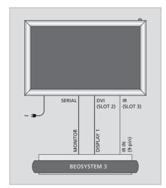
IR receiver: The screen has a built-in IR receiver. It is therefore not necessary to mount a separat IR receiver, as it is described in the BeoSystem Reference book. Only if a projector screen covers the built-in IR receiver when in use, you must mount a second IR receiver and connect it to the second IR-IN socket on your system.
